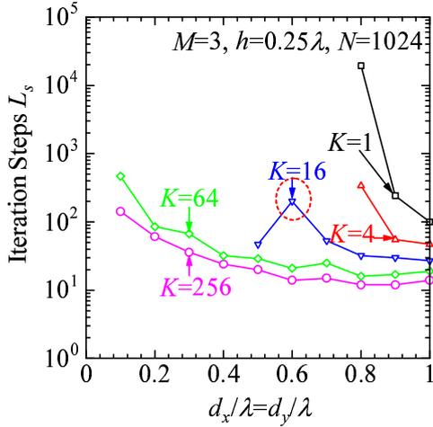
Figure 3: Required iteration steps versus array spacing.
