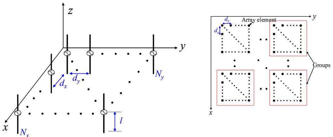
Figure 1: 2-D dipole array with  $N = N_x \times N_y$  elements.
