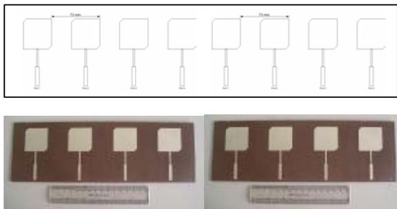
Figure 3 Layout and implemented 2.4 GHz array antenna
