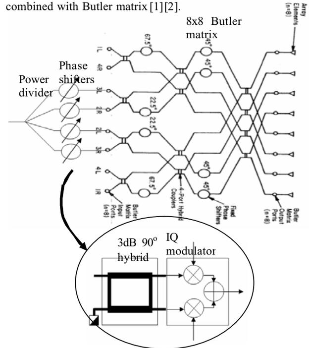
Figure 1 Low cost 2.4 GHz smart antenna configuration
