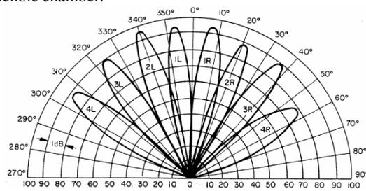
Figure 10 Simulated eight beams of Butler matrix only
