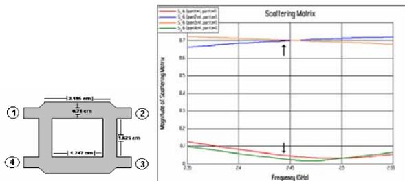
Figure 6. Hybrid 90° layout and its simulated S-parameters
