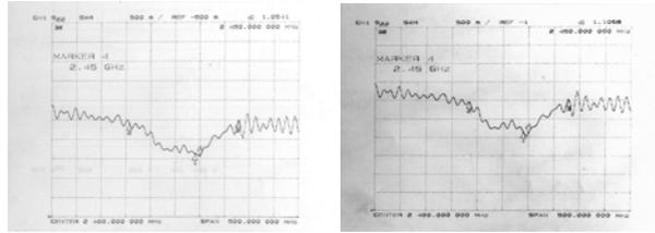
Figure 4 Measured VSWR of single patch and array antenna
