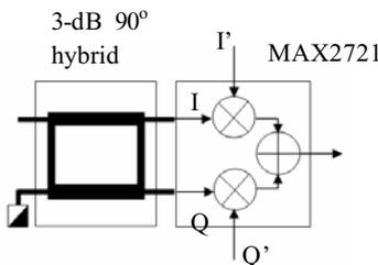
Figure 9 Block diagram of digitally controlled phase shifter
