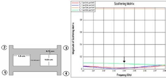
Figure 7. Cross over layout and its simulated S-parameters
