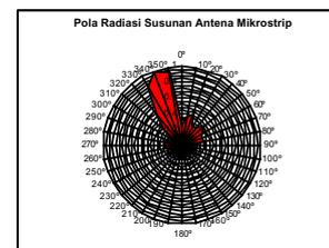
d) Measured of array beam of Butler matrix and phase shifters with phase differences -20°.
