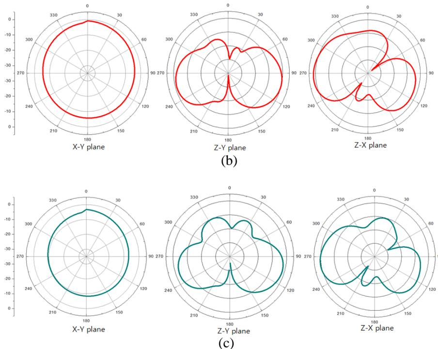
Fig. 6 Measured radiation patterns at (a) 849MHz, (b) 1920MHz, and (c) 2110MHz
