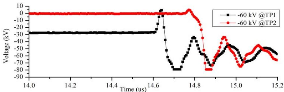
Figure 4: Breakdown delay with positive trigger pulse
