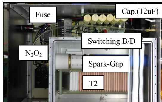
Figure 2: Structure of the implemented Trigger Generator
