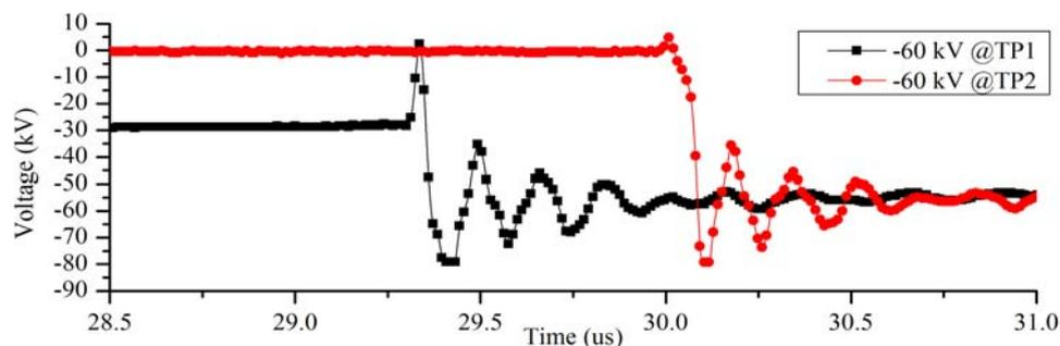
Figure 5: Breakdown delay with negative trigger pulse
