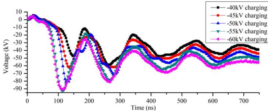
Figure 6: Comparison of the discharge time with different charging voltages
